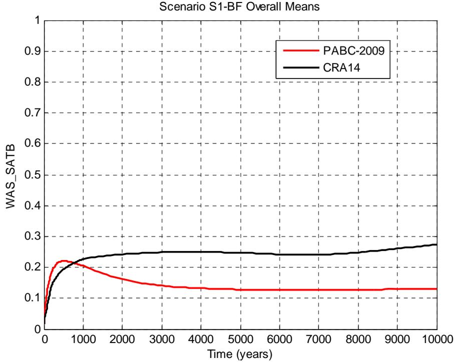
Figure 6-22: Overall Means of Waste Panel Brine Saturation, Scenario S1-BF.
