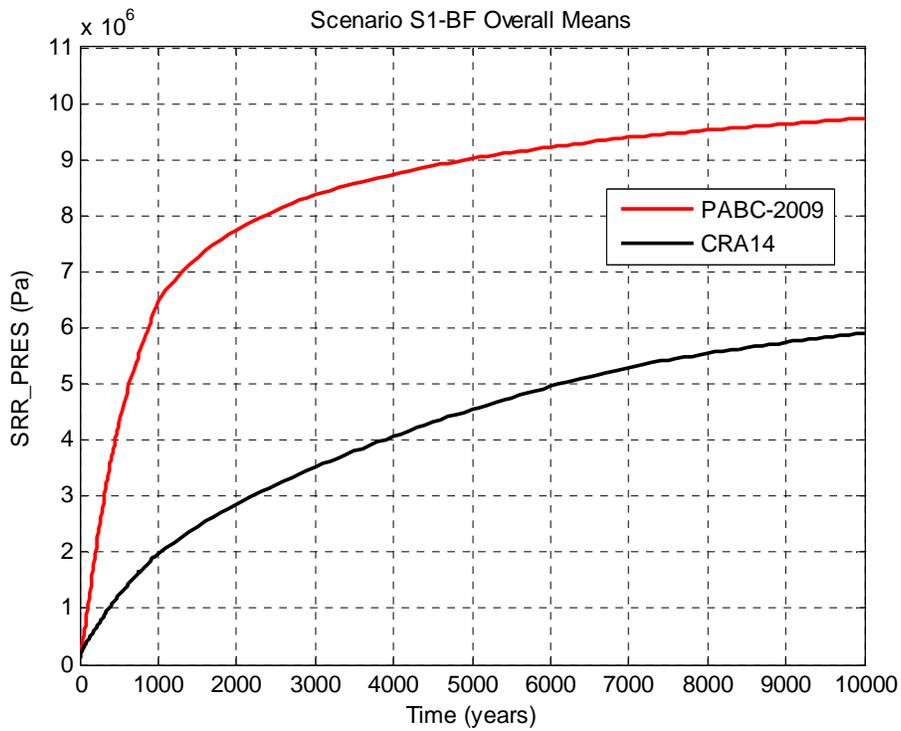
Figure 6-12: Overall Means of SRoR Pressure, Scenario S1-BF
